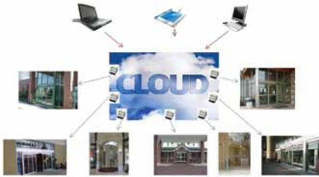
The Tormax iMotion Net is ideal for those customers who are concerned about the maintenance and performance of their automatic door systems. The Tormax iMotion Net provides for communication ready iMotion doors to be integrated into a building management system.
